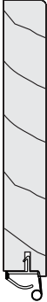
#39) Stationary Inside Stop with Weather Strip Right OXS (For 3 Wide Panel Units)
